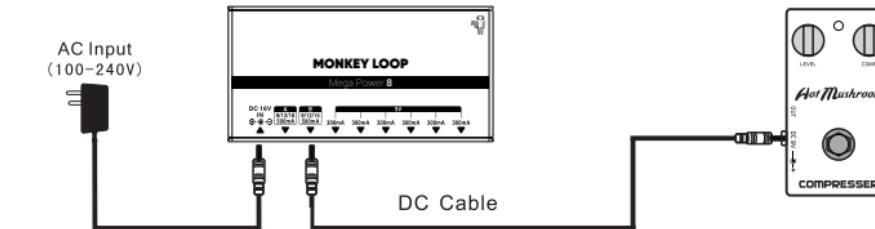
1. If the input polarity of the electrical device is
